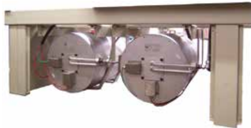
2 integrated NH 3 crackers
